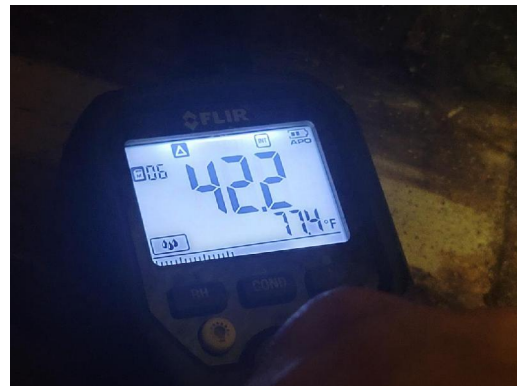
Interior Kitchen South lower wood framing Elevated moisture content (42.2%)
