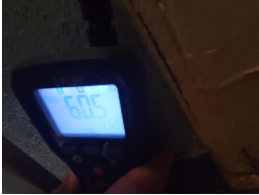
Interior East Bathroom West lower drywall Elevated moisture content (60.5%)
