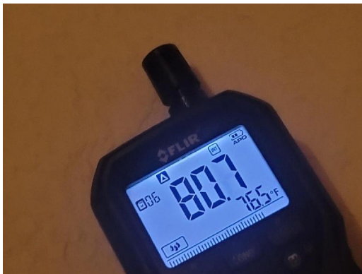
Interior West Bathroom West upper drywall wall Elevated moisture content (80.7%)
