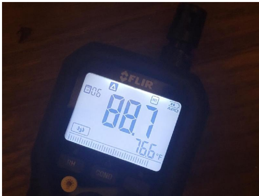
Interior Southwest Bedroom Northwest vinyl flooring Elevated moisture content (88.7%)
